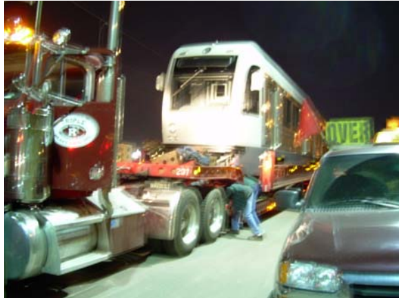
Triple R Truck is released and removed along with primary trailer unit.
