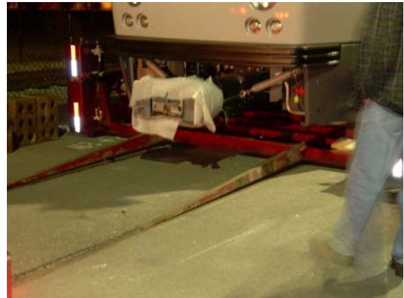
Roll off ramps are placed and aligned with track.
