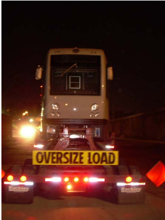
Trailer arrives at upper LA Gold Line site for unloading of P2550 / 705 seen here sitting on the new Hydraulic Trailer. (Trailers final unloading height is 6 inches from the ground.)
