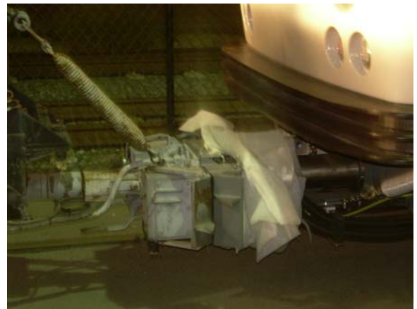
Tow vehicle connects with the P2550 / 705 and is towed into thy Gold Line Facility for inspection.
