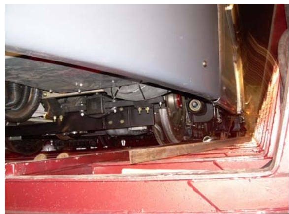
P2550 / 705 seated and secured on the custom trailer using chains and blocks through out the undercarriage and trailer.
