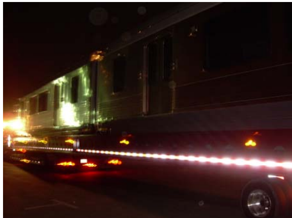
Trailer arrives at upper LA Gold Line site for unloading of P2550 / 705 seen here sitting on the new Hydraulic Trailer. (Trailers final unloading height is 6 inches from the ground.)
